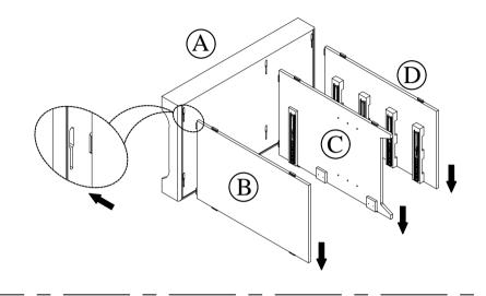
Step 3. Carefully align male and female bracket to connect left side panel B, right side panel D and partition panel C with front frame E, push the front frame E down to lock these panels in place.
