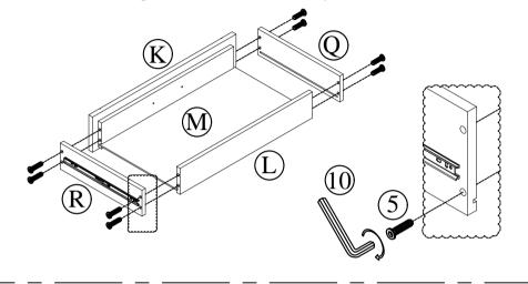
Step 12. Use bolt #5, allen key #10 to connect drawer side R with drawer front N and drawer back O, then insert drawer bottom P through lower channel on drawer front and back. Then use bolt #5, allen key #10 to connect drawer side Q with drawer front N and drawer back O to complete the drawer box assembly.
