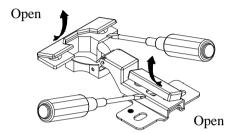
Step 7. Carefully hold the door I/J and make sure screw holes on door hinge base align with predrilled screw holes on inside of partition/side panel, use philips head screw driver and screw #7 to attach door hinge #6 on inside of partition/side panel. Adjust the screw on center portion of hinge slightly by loose or fasten screws to make sure even gap around door, and close the 2 covers on the door hinge #6.
