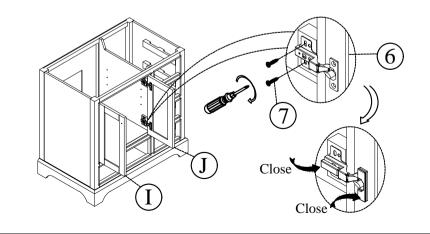
Step 6. Make sure screw holes on door hinge align with predrilled screw holes on backside of door panel, use philips head screw driver and screw #7 to attach door hinge #6 on backside of door panel I/J.
