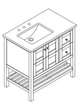
Step 15. With the vanity in its location and all plumbing in place, apply a bead of silicone to the unpolished back side and bottom edge of the backsplash and secure it to the vanity. Wipe away any excess silicone immediately. Allow 24 hours to dry.
