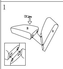
Step 1:Carefully align the male B and female metal A bracket then push all the way down to secure seat and back connection.
