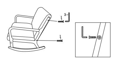
Step 3:Connet the chair frame (finished in step 2) and the seat body (finished in step 1). Align the screw hole at the frame of chair and seat backrest, screw in the bolt 1, washer with Allen Key 3.
