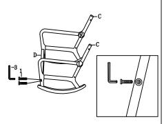
Step 2:Connect the armrest C and Rung D.
