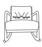
Use hands to push the seat cushion to balance the chair, then sequentlly tighten the screws till are fully tightened  $_{\circ}$
