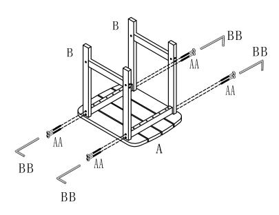
**STEP 2:** Use bolt AA, allen key BB to attach bottom stretcher C with legs B, make sure all parts properly connected and aligned then fasten all bolts to secure. Turn the whole table upright. Assembly completed.
