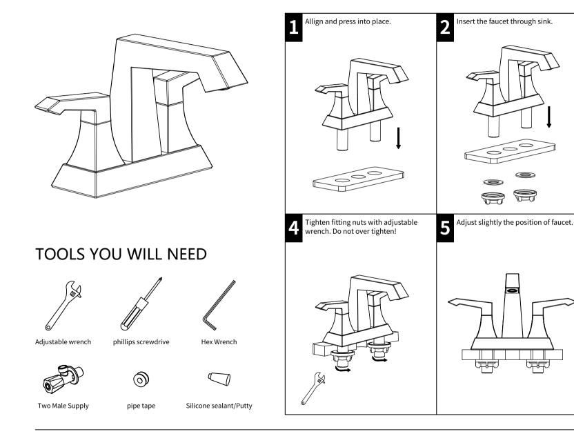
ring and the sink. P Connect and tighten the supply hoses. 6
