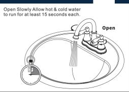
**CONFIRM PROPER INSTALLATION**
